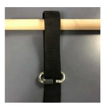
Step 2: Feed ring end of strap into quick link as shown.
