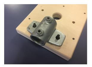
Place flat washers over each screw, followed by lock washers, then hex nuts. Tighten down hex nuts.
